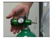
3. Open the cylinder by turning the valve wheel counter-clockwise until the gauge shows contents.
